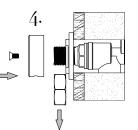
Remove Gauge and insert Handle Adapter (4) and screw tight (3).
